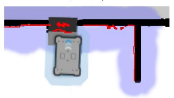
5.1. The red lines represent what the laser scanners see. The robot is correctly localized when they align with the black lines that represent walls.
