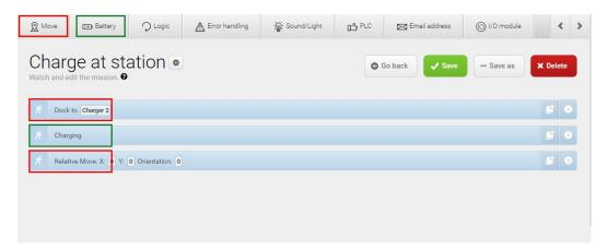
The next steps describe how to set the parameters of the chosen mission actions. To set the parameters of each action, open the action dialog by selecting the gearwheel icon of the action in question.
