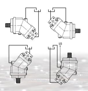
In installations where the position of the pump is above the tank, ensure the drain line is always underneath the fluid level tank.
